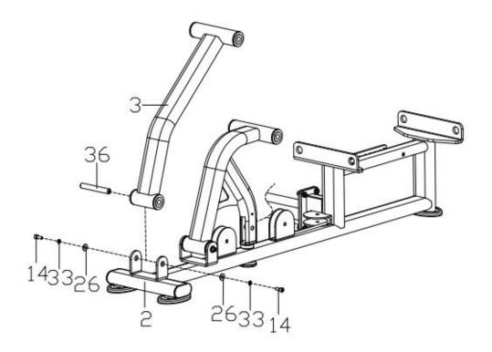
Step 5 Attach the footrest (5) to the frames (3 and 4) with bolts (14), washers (33 and 26) and shaft (37). Tighten all previous bolts (14).
