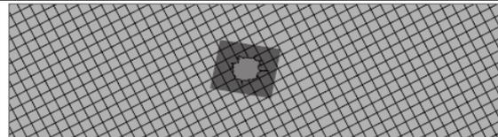
4. Stick and press onto the vinyl patch. Do not inflate for at least 20 min.
