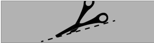
1. Cut the repair patch according to the size of the puncture.
